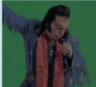
Picture too dark on all channels. Slowly adjust either the brightness or contrast control.
